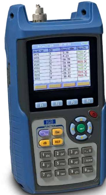
AE700 is a DWDM Channel Analyzer for the installation and maintenance of DWDM systems. The handheld unit is able to measure wavelengths in the c-band, which is from 1530 to 1565 nm. The AE700 also supports optical signal to ratio (OSNR) which is essential for verifying signal quality. The measurements can be displayed in both graphical or list formats.
