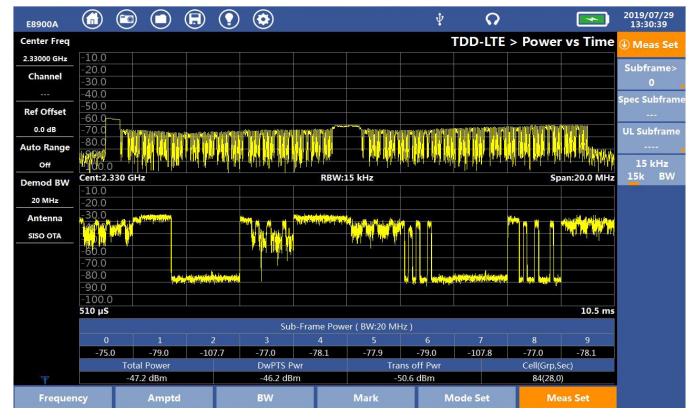
Figure 4: TDD-LTE power vs. time measurement.
