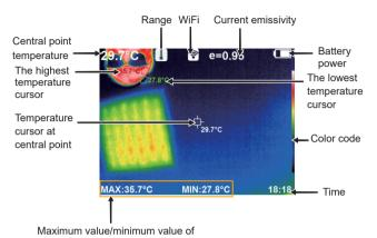
Range: The range of temperature measurements.
