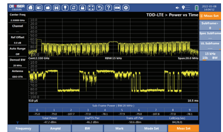
Figure 6: LTE Power vs Time chart provides both time-domain and spectrum analysis.
