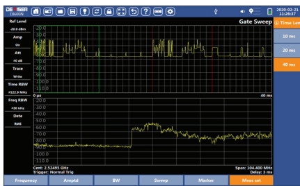
Figure 4: Gated Sweep provides specific slot spectrum of a TDD system.
