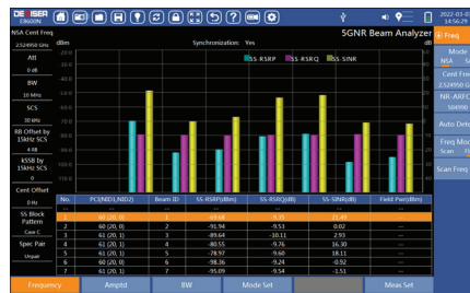
Figure 5: 5G NR beam analysis measures up to 8 beams at once.
