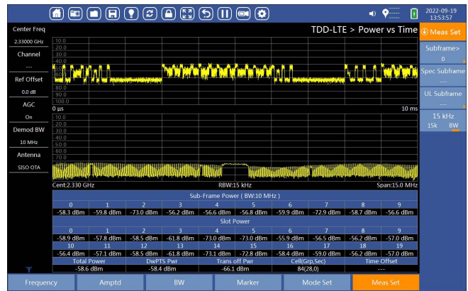
Figure 4: TDD-LTE power vs. time measurement.
