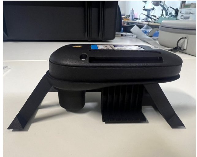
Personal monitor secured on the fixture (side view)
